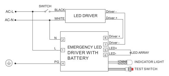
1.DO NOT MATE CONNECTOR UNTIL INSTALLATIONIS COMPLETE AND AC POWER IS SUPPLIED. 2.TEST ACCESSORY LEADS-OBSERVE PROPER POLARITY WIRING.
